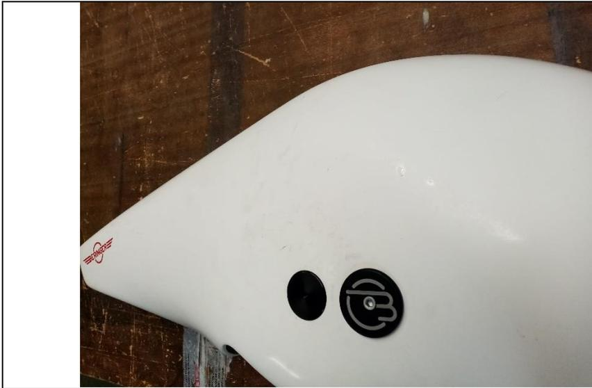
Push into position the valve access cap BCH-010.
