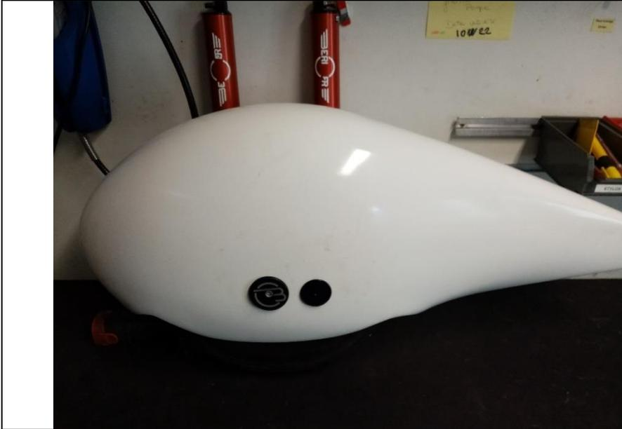
Push into position the valve access cap BCH-010.
