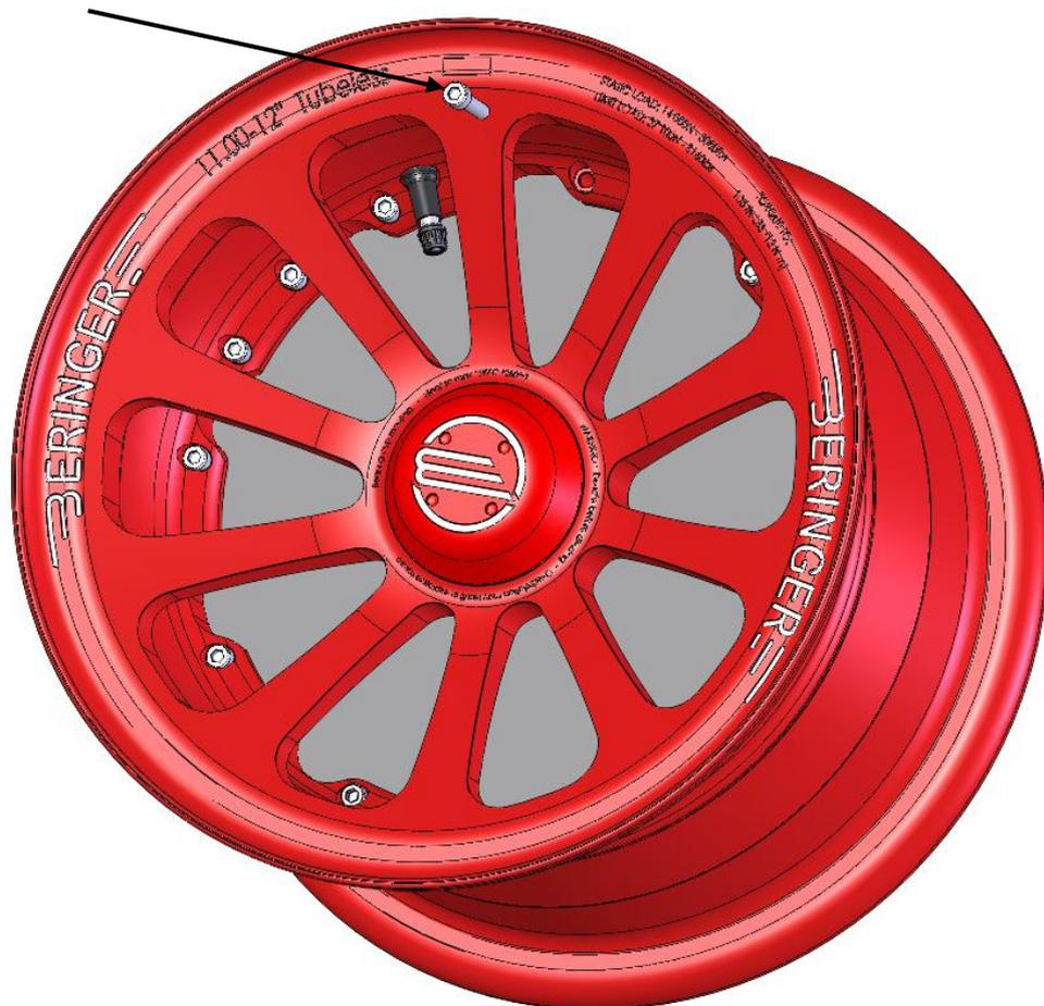
4. Check the length of the screw is 30mm (thread only). If not, replace it with a V-CHC-009 with correct length of 30mm
