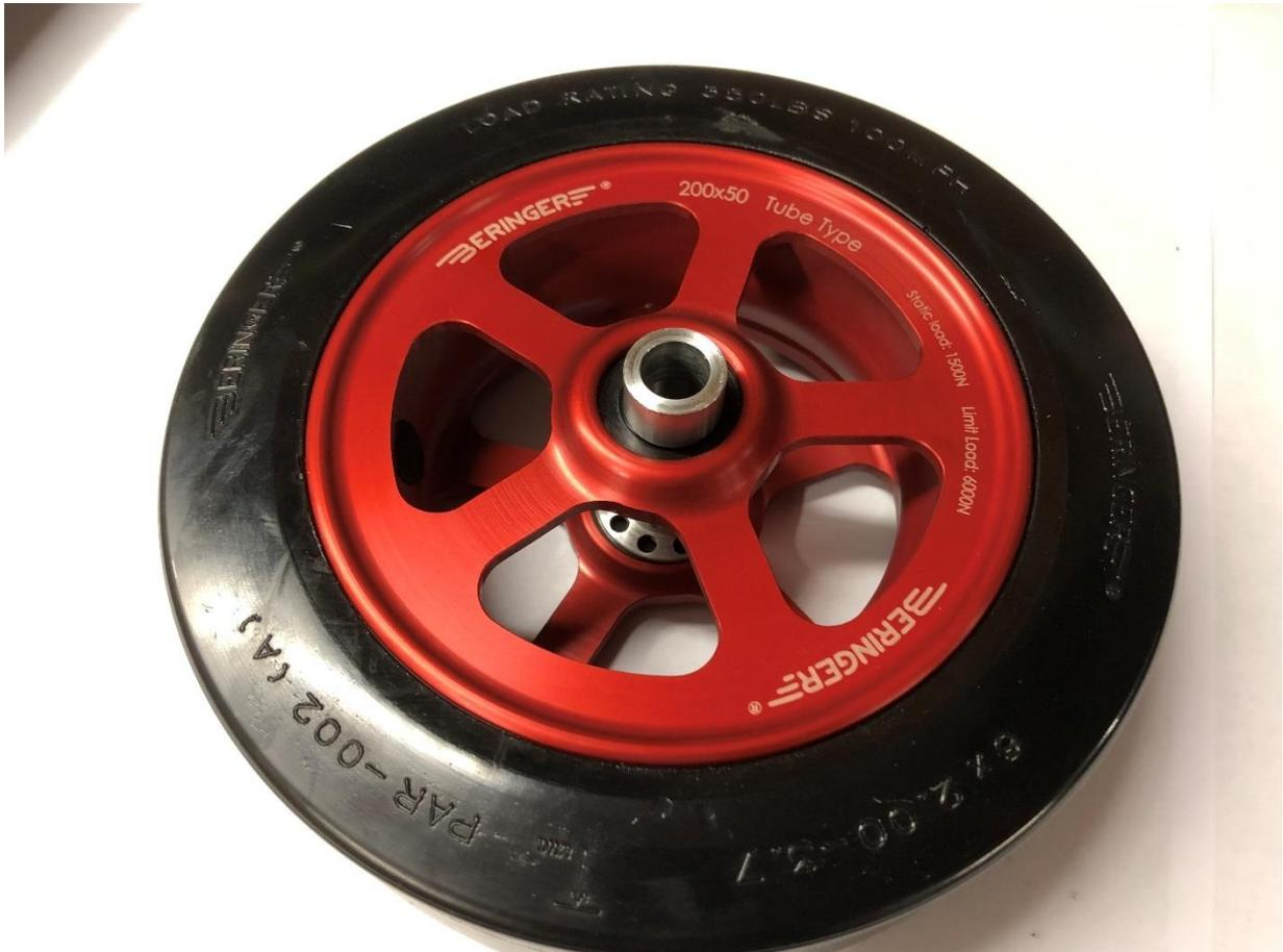
10. To finish installation of the tail wheel please refer to aircraft manual to respect torque etc.
