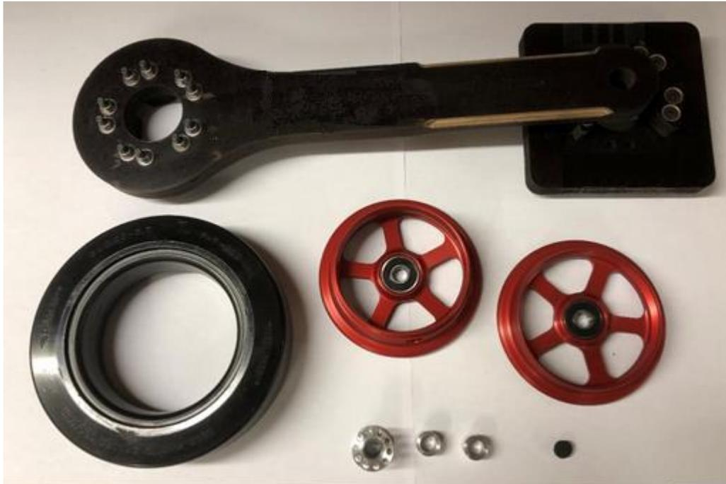
2. Position the plastic plug into the valve hole, by pushing it from the outside towards the bearing. Dimple towards the thread.
