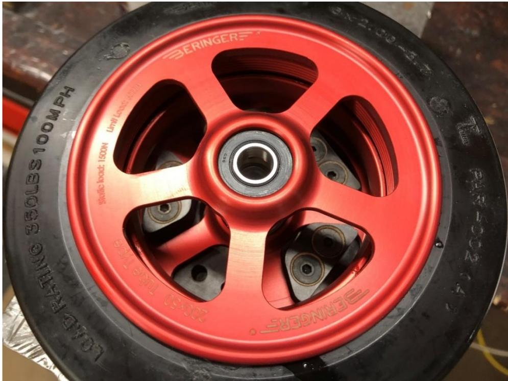
8. Using the spanner tool screw the rim to a complete stop by applying good force to push the tool down.
