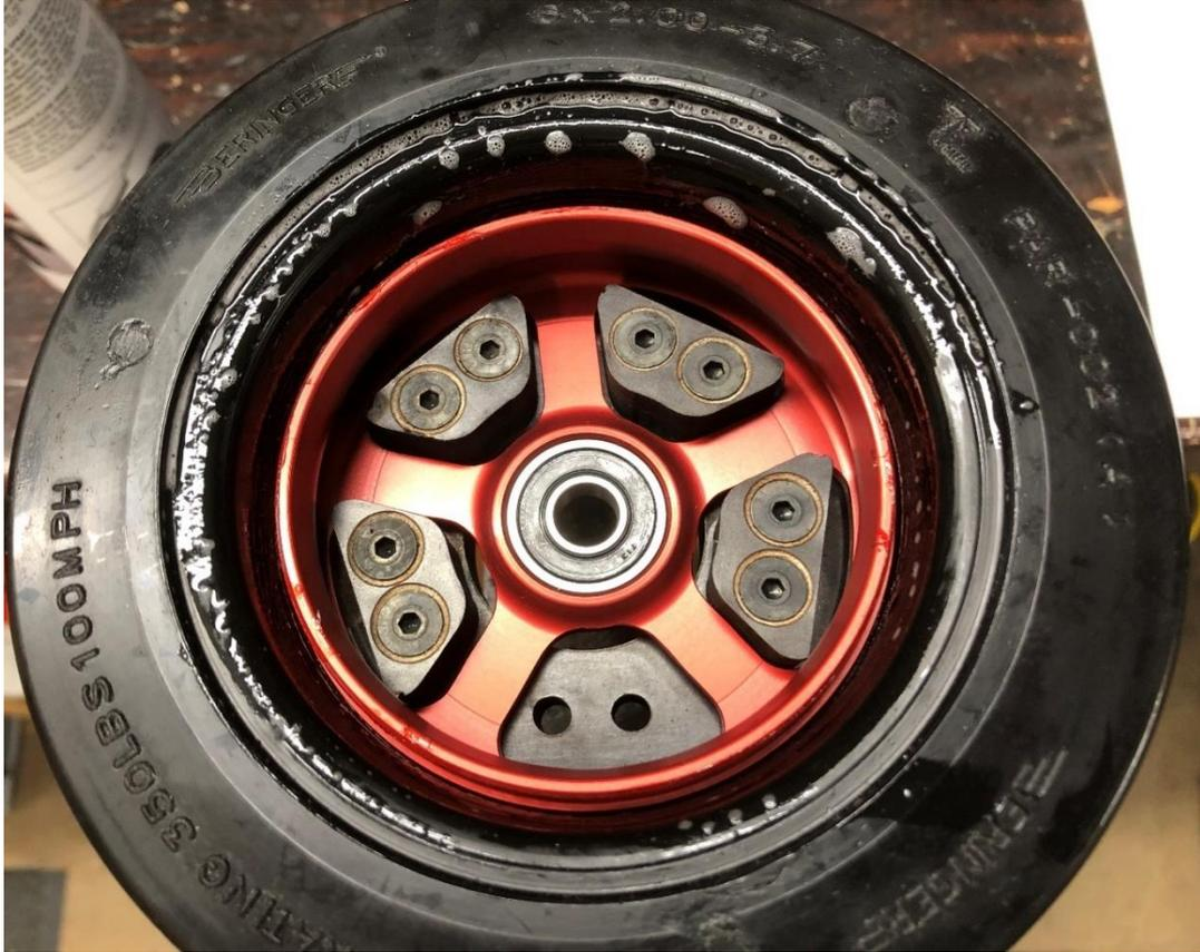
6. Place into position the aluminium spacer as shown below.
