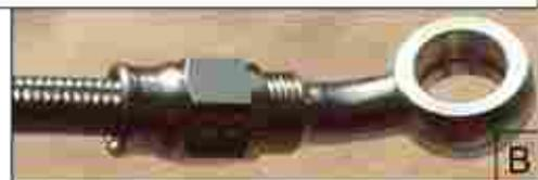
6- Finish tightening the socket onto the fitting :
