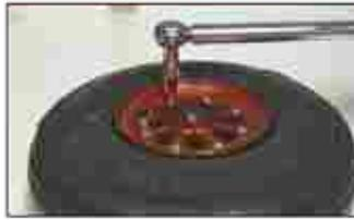
Torque tighten to 10N.m (+-1Nm) equivalent to 1m.kg (+-0.1m.kg)
