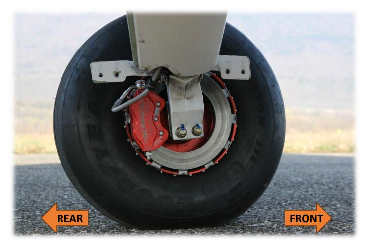
Brake caliper shall be installed ideally with bleeding screw facing downward and if possible on the rear side of the wheel
