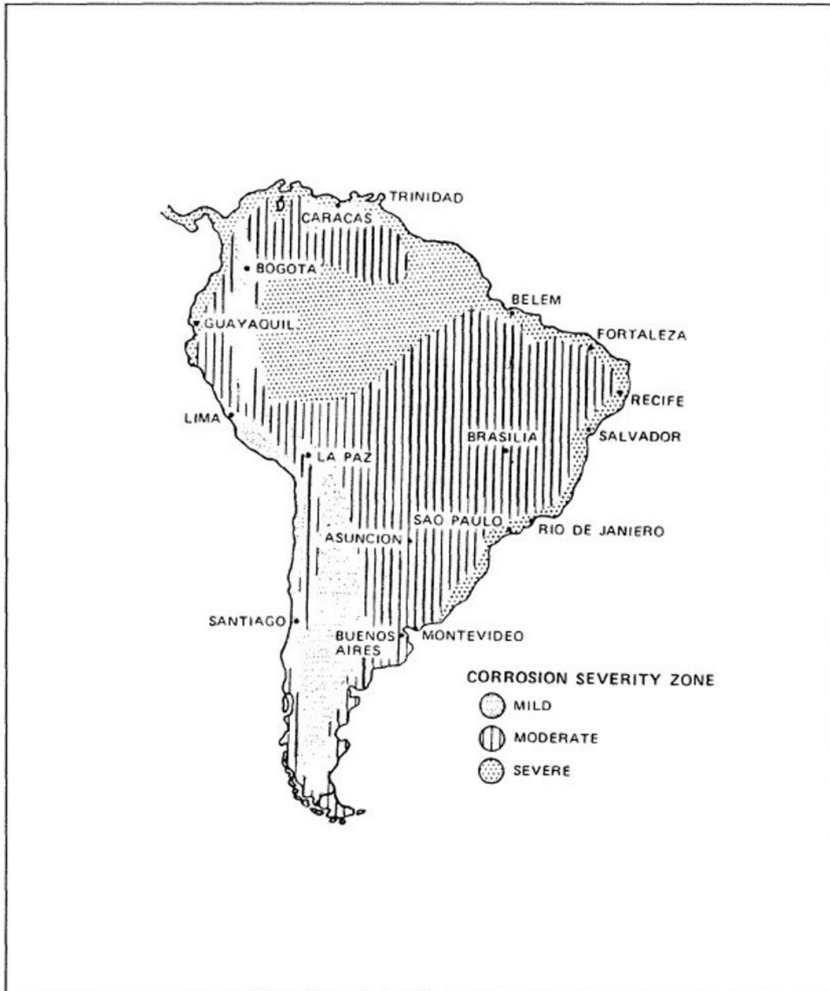
Figure 4-16. South America Corrosion Severity Map
