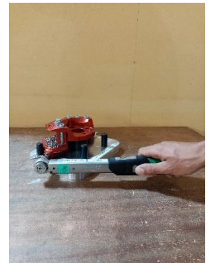
3 Torque / Couple 5 N.m (44in.lbs) + 90°
