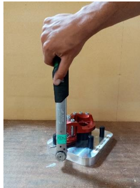
2 Torque / Couple 5 N.m (44 in.lbs)
