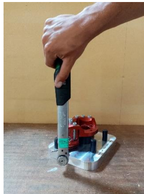
2 Torque / Couple 5 N.m (44 in.lbs)
