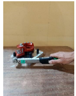
3 Torque / Couple 5 N.m (44in.lbs) + 90°
