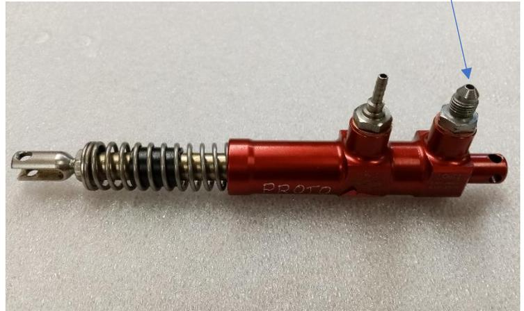
Note: Unlike the standard procedure, the pressure is applied at the reservoir. This procedure is recommended for pilot & copilot master-cylinder configuration.
