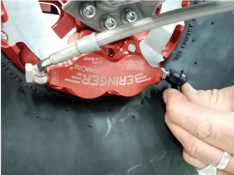
Plug the pressure bottle to the bleeding screw of the caliper
