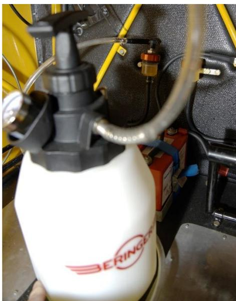
Remove the reservoir cap and membrane and replace it with the one furnished with the bleeding kit. Connect the pressure bottle to the cap. (double check the membrane is pierced to allow fluid flow for the bleeding). Make sure the bottle is filled with fluid with at least 400 ml (14.1 oz).
