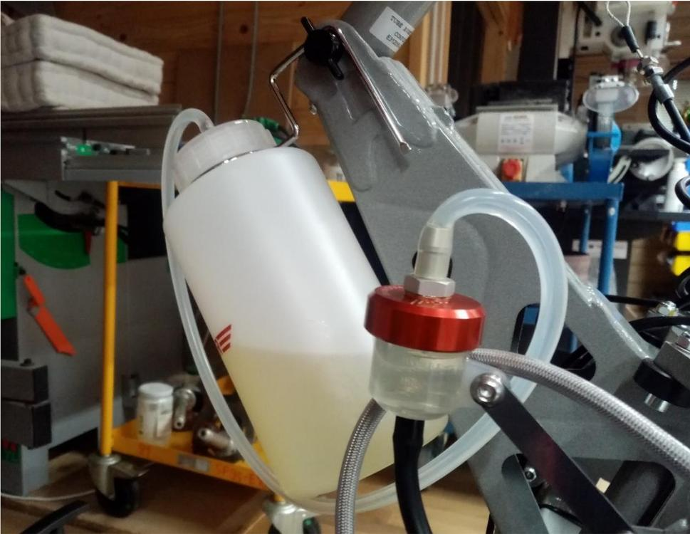
Ensure there is no more bubble circulating before closing the circuit by screwing the bleeder screw on the caliper
