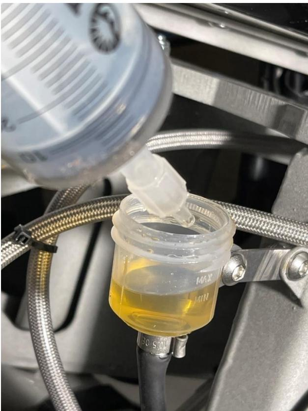
If necessary, remove fluid from reservoir using
