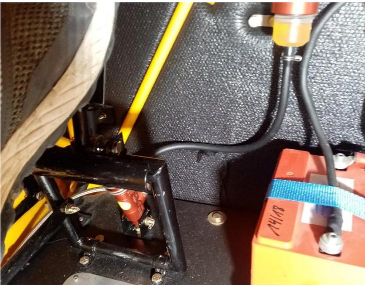
While bleed screw is still open and fluid is flowing through system, fully depress then slowly release the pedal / lever 3 times
