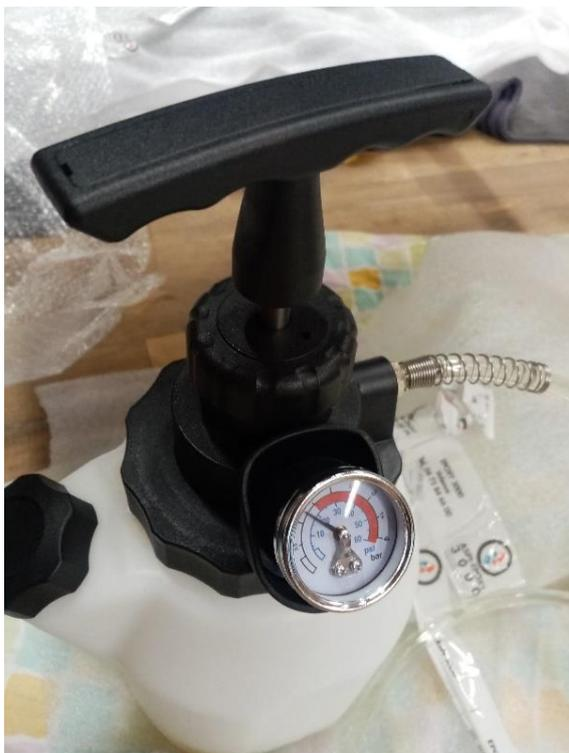
Close the pressure bottle and inflate it to 1.2-1.5 bars (17-21 psi) and open the caliper bleeding screw
