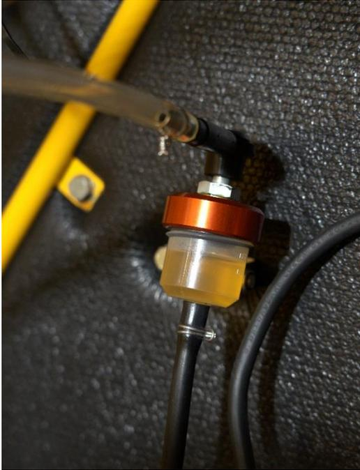
Let the fluid flow until there is no bubble seen in the hose, be careful not to pass all fluid and reinject air
