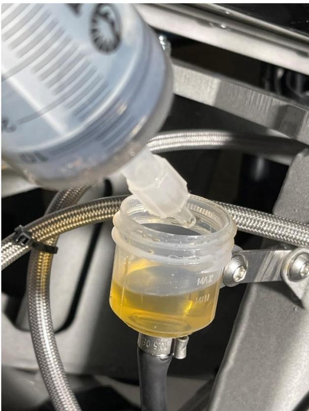
If necessary, adjust fluid level from reservoir using a syringe or a rag (lower the fluid level by about 5mm / 0.2" (from the top, below Max level indicated)
