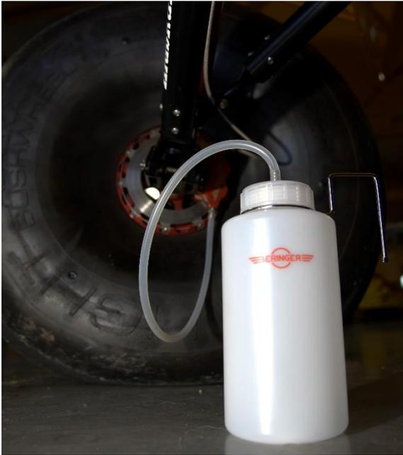
Connect the catch can to the bleeding screw of the brake caliper
