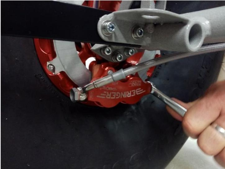
Unscrew bleeding screw and let the brake fluid flow in the reception bottle until there is no more bubbles appearing in the circuit
