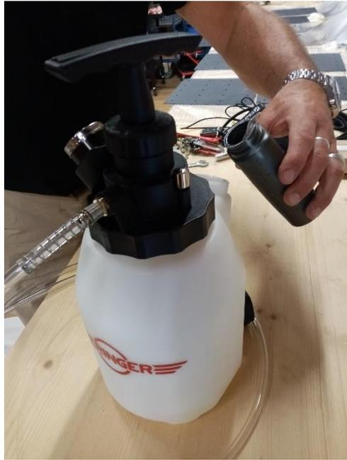
Fill the pressure bottle with the brake fluid
