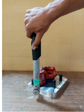
2 Torque / Couple 5 N.m (44 in.lbs)
