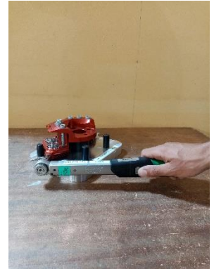
3 Torque / Couple 5N.m (44in.lbs) + 90°
