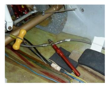
j) Secure the limiter with straps and foam so it cannot move.
