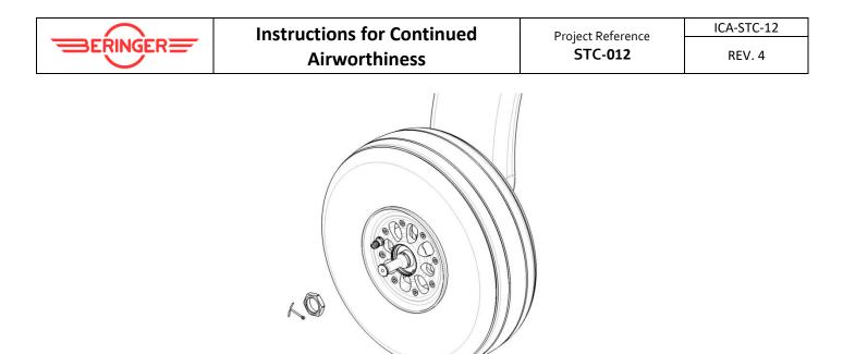
j) Place the safety wire (stainless steel 1mm – 0.040") in the ring groove all around the wheel.CAUTION: This safety wire must be in place to secure the disc.
