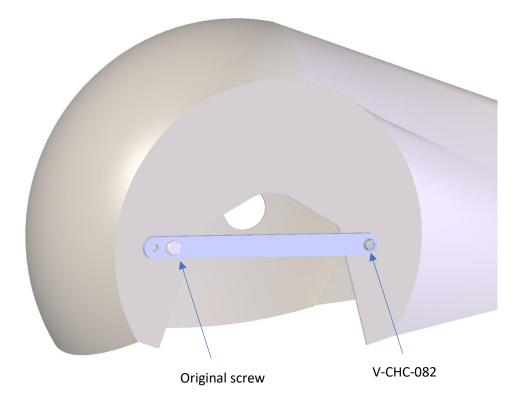
5- Drill the new fairing fore hole with  $\frac{1}{4}$ " (6.35mm) drill
