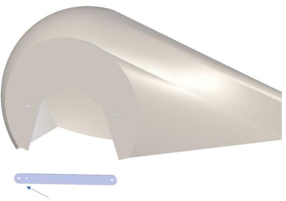
Side with two holes aft of the aircraft
