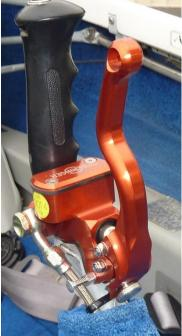
e) Check carefully that the lever is not touching anything when moving the stick in all positions
