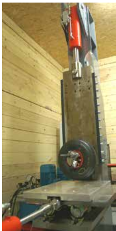
← ↑ 440,00lbs Hydraulic press for ultimate load tests Roll tests : 29" tires →
