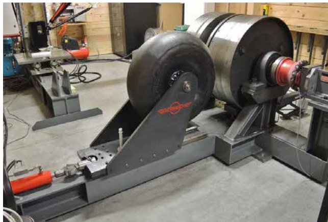
← ↑ 440,00lbs Hydraulic press for ultimate load tests Roll tests : 29" tires →
