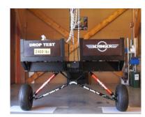
The patented ALG landing gear had to go through several tests for the certification process (FAA-EASA)
