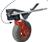
Locked: the connection wheel/ rudder is riaid with a freedom of +/-20° (steering is done with the rudder pedals)
