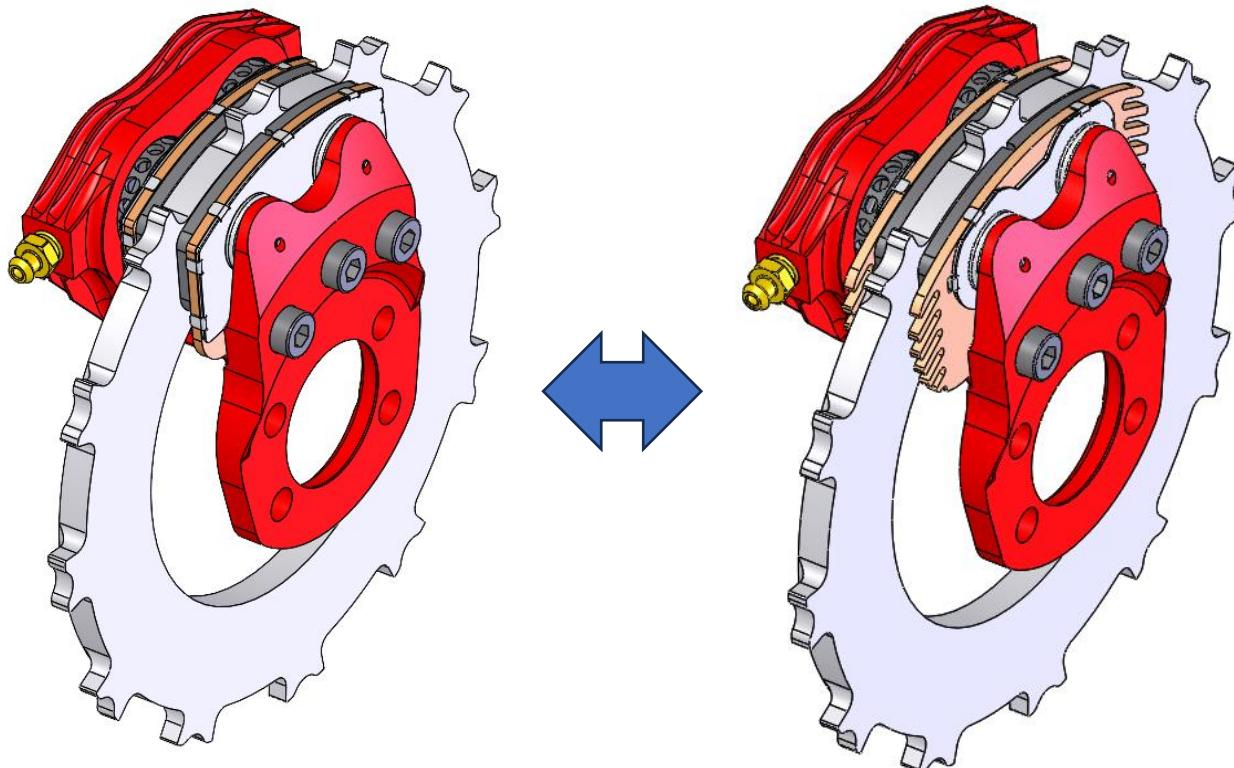
New brake pads PQ-110.2 and PQ-110.1 are interchangeable with the previous PQT-010 and are available as spare parts for the Legacy calipers.
