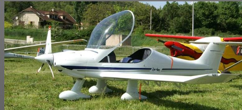
The MCR of JB Duchatelle equipped with the 3 wheels and pedal brakes (pilot & co-pilot) and the ALIR anti-skid plus parking brake valve.
